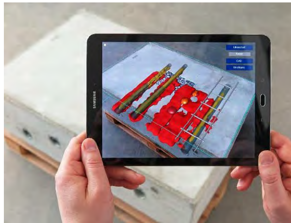
Figure 5: Augmented Reality visualization using a tablet: Tablet showing the AR-app, the test specimen, and the optical marker.
